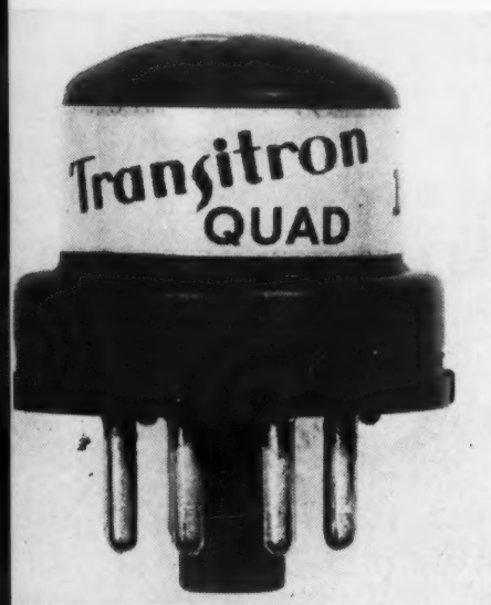
Fig. 2. The diodes are available in matched quads or pairs mounted in either octal bases (top) or 7-pin miniature bases (bottom).
